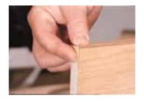
To trim the edge, start by carefully bending over the ends until the veneer breaks. Make sure you apply pressure to the end of the attached veneer so it doesn't splinter back onto the visible edge. Then pull the "dangling chad" of veneer downward to tear it free. By the way, if you're doing four edges of a board, do two opposite edges first, trim the edges, then apply the other two edges.
