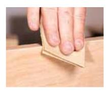
TThe file is too aggressive for a finished edge, so trade it in for some 220-grit sandpaper and finish cleaning up the edge. You'll find some of the adhesive is stuck to the face of the board. This can be lightly sanded off, but proceed carefully to avoid sanding through the face veneer. That's all there is to it, but don't go using the clothes iron, buy your own for the shop!
