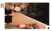
Once the two side wedges are cut to rough size, trim them a little closer to accurate on the jointer. Once you're within about 1/16" of the finished line, clamp the boards together and get out a bench plane. With a little hand work the pieces will match up perfectly.
