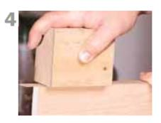
Since trying to use the iron to hold the tape in place as the glue dries just re-heats the glue, switch to a simple block of wood. The chunk of poplar shown here works great. The bottom surface is sanded smooth and the edges are broken to avoid snagging or scratching. Simply apply pressure and make long passes over the edge for about 30 seconds. If you have a few pieces to veneer, set the first piece aside for now to let the glue cool.
