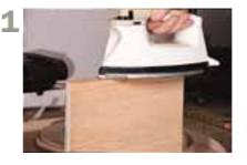
These first six photos show the sidebar "Iron-on Wood" below. Start with a piece of tape that's about 2" longer than the edge you are covering. Your iron should be on a cotton setting, with the steam turned off. Make sure the tape overhangs the edge evenly, then start ironing. Make long passes over the edge, not stopping in any one place for any length of time, applying heat evenly. The tape will start to curl up a little as the glue melts.
