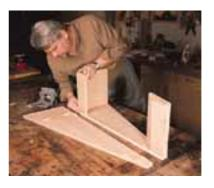
With all the cross members cut, the biscuit joiner makes it possible to pull the project together. This photo also shows the two cleats in place at the top and bottom of the
